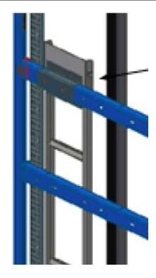
An additional structure ring member will be provided with an extra guide plate as seen in the photo above.
